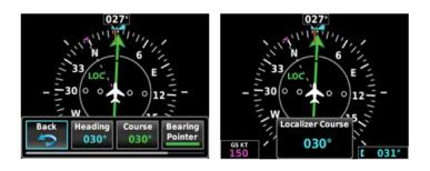
Up to two single needle bearing pointers can be displayed on the HSI. These are also selected from the menu. The options are GPS1, VOR1 (NAV1) and VOR2 (NAV2). It is not possible to display ADF data, but displaying the GPS1 bearing pointer and routing direct to an NDB on the GTN750 would provide a similar presentation.
