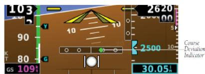
When GPS is selected, the CDI bar is automatically set to the desired track (DTK) for the current flight plan leg. There is no need to manually adjust the CDI bar.
