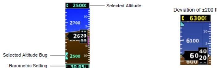
The altitude alerting function is active at all times and could be particularly useful when flying manually in proximity to controlled airspace. A deviation alert is provided when  $\pm 200$ ft from the selected altitude, so flying at least 300ft below the base of controlled airspace and selecting or synchronising this altitude would provide a warning before infringement.
