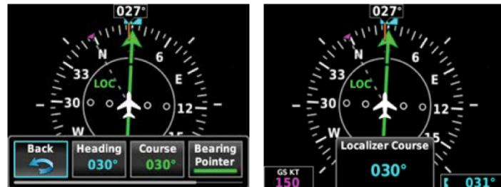
Up to two single needle bearing pointers can be displayed on the HSI. These are also selected from the menu. The options are GPS1, VOR1 (NAV1) and VOR2 (NAV2). It is not possible to display ADF data, but displaying the GPS1 bearing pointer and routing direct to an NDB on the GTN750 would provide a similar presentation.
