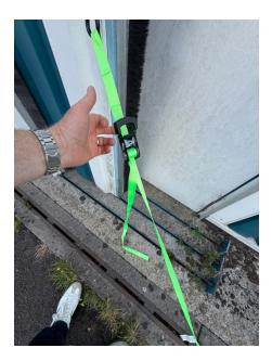
To release, pull the inner handle upwards and rotate the main rachet until it's almost 180 degrees as shown below. Then you can pull firmly on the strap and the drum will unwind. If it isn't unwinding you haven't got the rachet handle far enough, it's quite stiff for the last 15-20 degrees.
